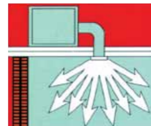
Side discharge roof installation
